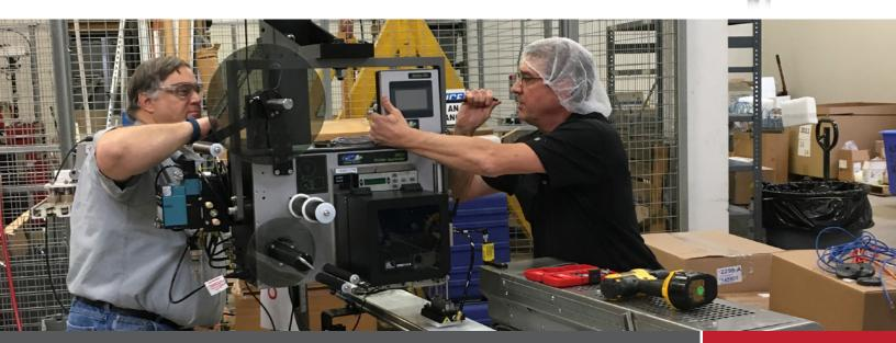
custom logos and assorted bar codes. The CTM 3600a-PA can also accommodate labels up to 7.1" wide and features a user-friendly interface, tamp-blow operation and operator keyboard and display.
